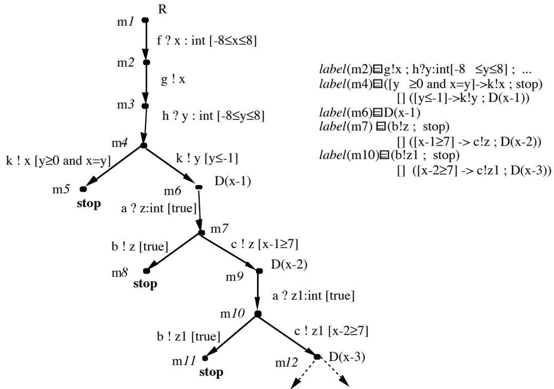
Fig. 1 An Extended Labeled Transition System  $ELTS(t_1)$  for LOTOS Expression  $t_1$
