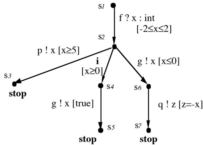
Fig. 2 An Extended Labeled Transition System  $ELTS(t_2)$  for LOTOS Expression  $t_2$
